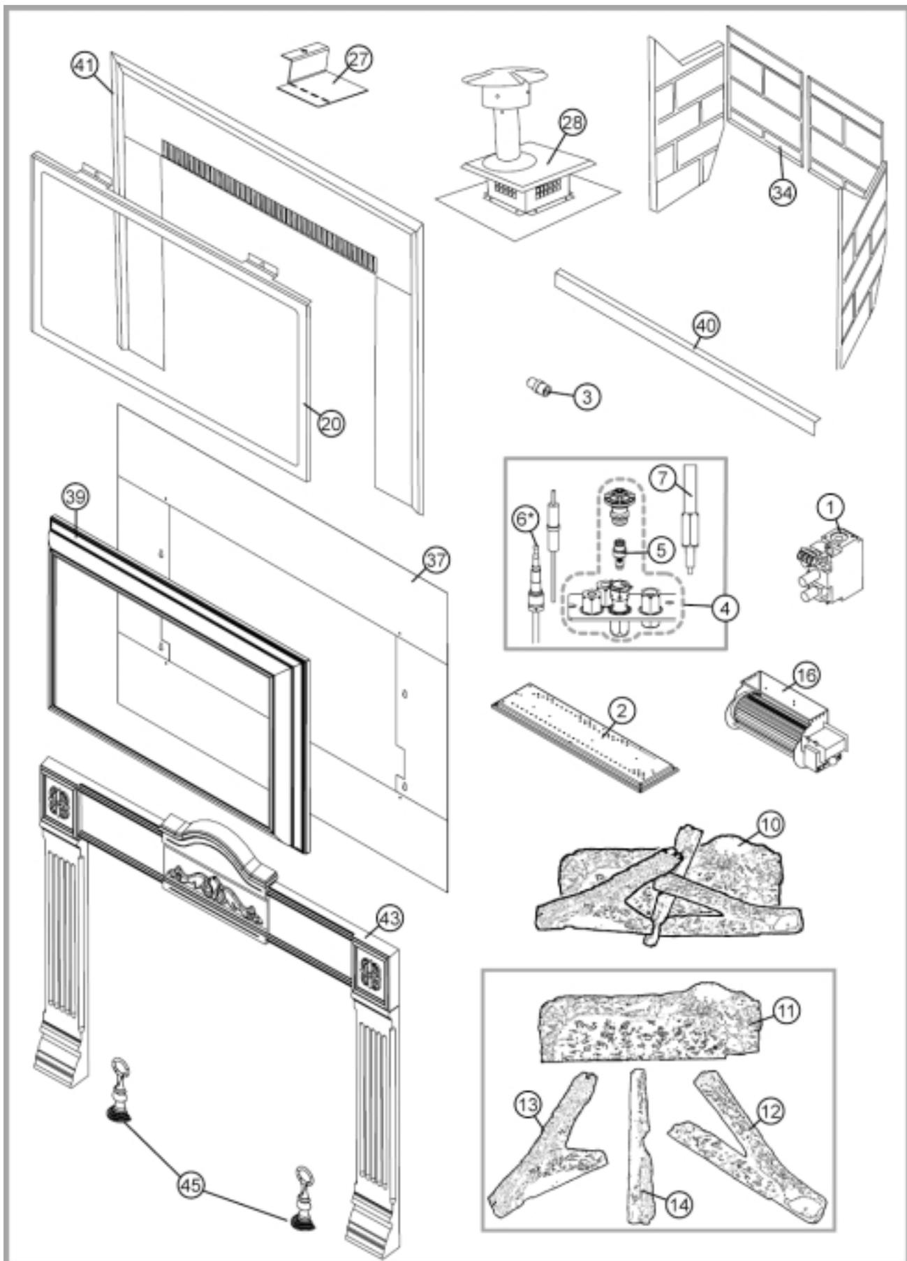
\* **WARNING:** This is a fast acting thermocouple. It is an integral safety component. Replace only with a fast acting thermocouple supplied by Wolf Steel Ltd. W415-0223/D/01.12.04
