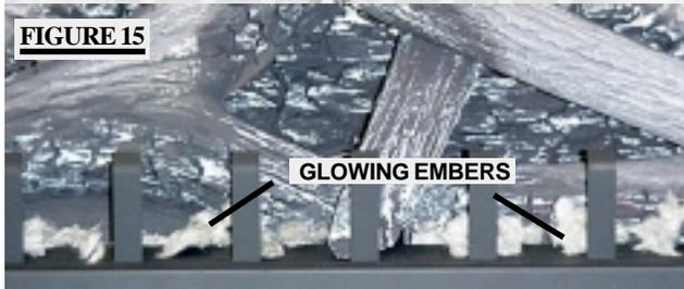
4. Tear the glowing embers into pieces and place along the front row of ports covering all of the burner area in front of the logs. Care should be taken to shred the embers into thin, small irregular pieces as only the exposed edges of the fibre hairs will glow. *The ember material will only glow when exposed to direct flame; however, care should be taken to not block the burner ports.* Blocked burner ports can cause an incorrect flame pattern, carbon deposits and delayed ignition.
