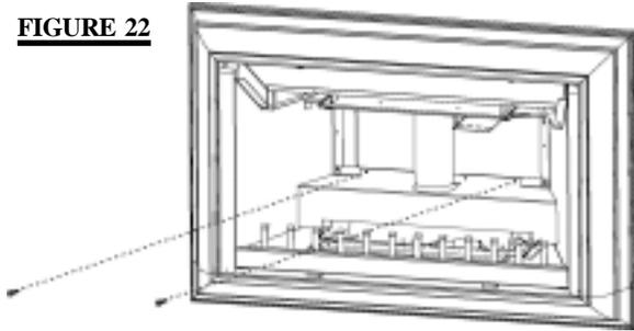
3. Detach the two screws from the back of the firebox and remove the panel, as illustrated.
